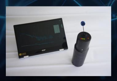
γ Tube20x is controlled manually or automatically and remotely to reduce the dosimetric impact of operators. It is a versatile tool, both designed for nuclear spectrometry experts and radiation protectionists.
