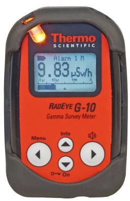
The RadEye G is a light-weight and very rugged instrument designed for quick and reliable measurement of gamma dose rates. Modern electronic circuitry guarantees excellent linearity over 6 decades of radiation intensity: from background level to 10 R/h - with overrange indication up to 1000 R/h. The RadEye G-10 version incorporates a different energy filter in order to achieve a Sievert response curve according to ambient equivalent dose rate H\*(10).
