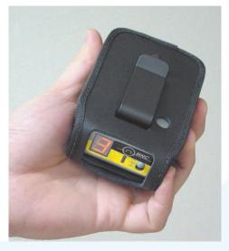
The unit fits inside a protective pouch and secures to the belt of the user while in operation or for transportation.
