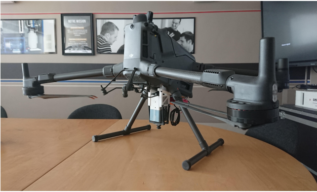
Fig. 1. Complete UAV-detector assembly (DJI Matrice 400 with H3D M400i payload).
